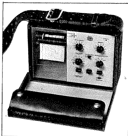
Fig.3. The portable Level Recorder Type 2306
